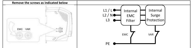
The Optidrive product range has input supply voltage surge suppression components fitted to protect the drive from line voltage transients, typically originating from lightning strikes or switching of high power equipment on the same supply.
